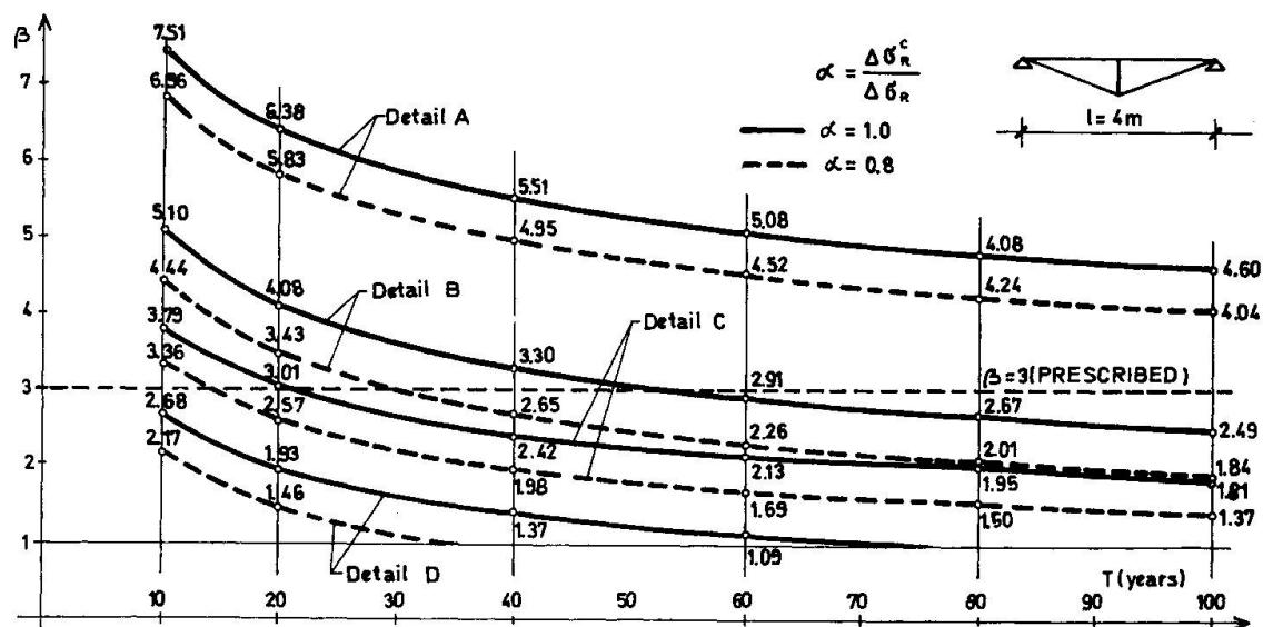
Fig. 5 Durability decrease at corrosion fatigue ( $\alpha = 0.8$ )
