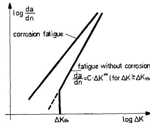
Fig.2 Corrosion fatigue expressed by
