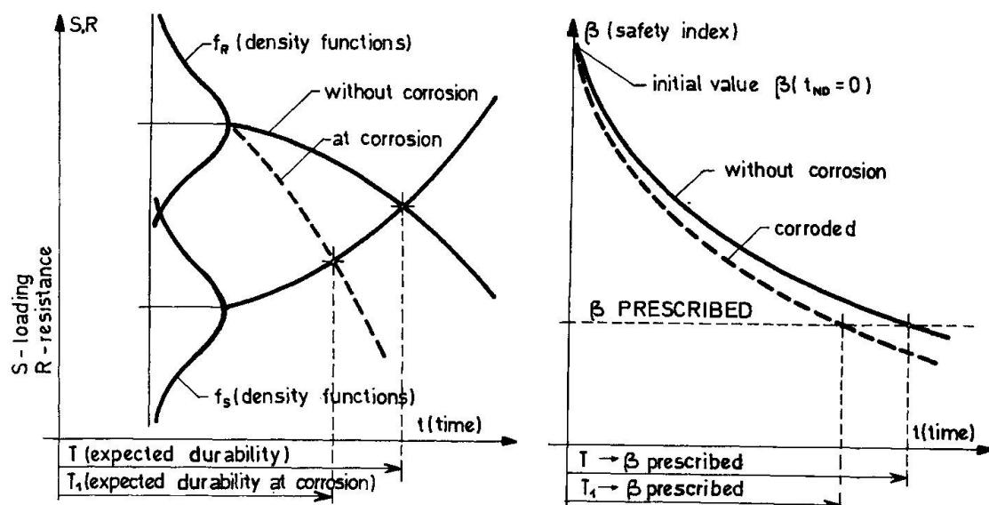
Fig. 3 Relation of reliability and durability at corrosion fatigue
