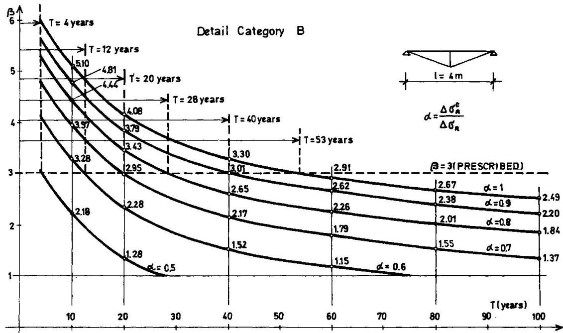
Fig. 6 Durability decrease of detail B for various coefficients
