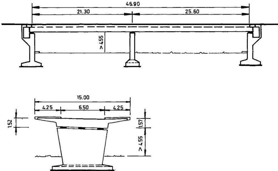
Fig. 3 Longitudinal section and cross section of Bridge Ulenbergstrasse
