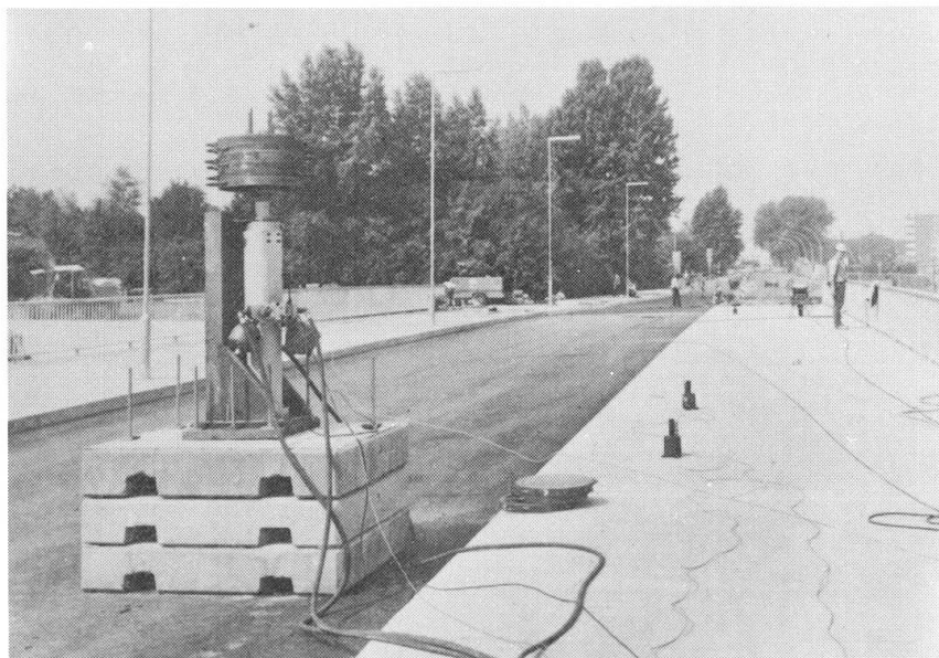
Fig.1 Hydraulic actuator and transducers on Bridge Ulenbergstrasse
