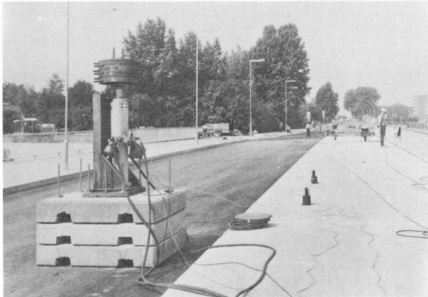
Fig.1 Hydraulic actuator and transducers on Bridge Ulenbergstrasse
