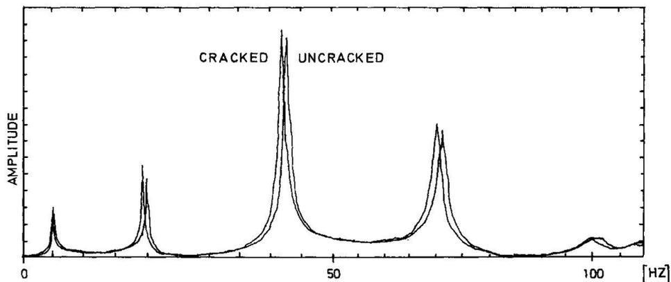
Fig. 2 Transfer functions of the test beam
