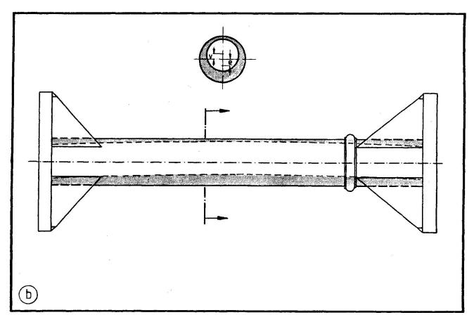
fig. 8 Cast-iron hollow columns with varying wall thickness due to slipping of the mould core.
