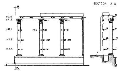
Fig. 5 - Vertical view of sensors and vibrodyne locations.
