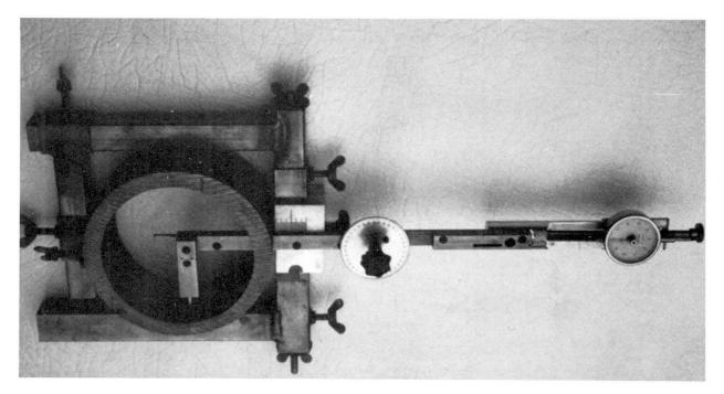
fig. 10 Mechanical wall-thickness-measuring-device.
