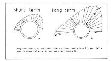
Fig. 5 Diagram of the soil-liner interface pressures at short and long term.
