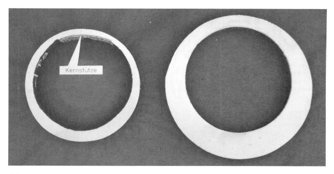
fig. 9 Cross sections of cast-iron hollow columns.
