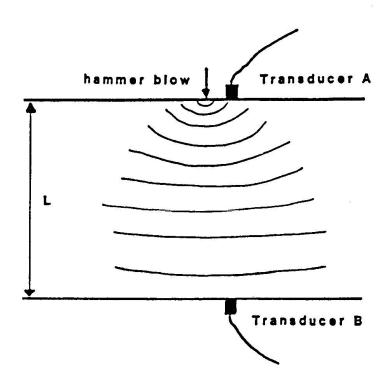
Fig. 1 Time Delay Technique
