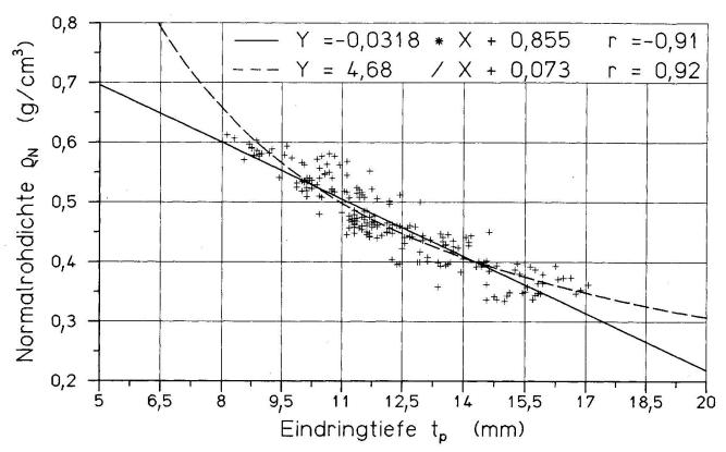
fig. 6 Relationship between density and Pilodyn 6J penetrations in spruce (Piceae abies). + = average of 16 measurements.
