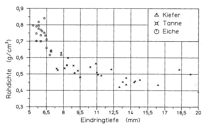
fig. 7 Relationship between density and Pilodyn 6J penetrations. Oak, pine and fir from the 18th century.
