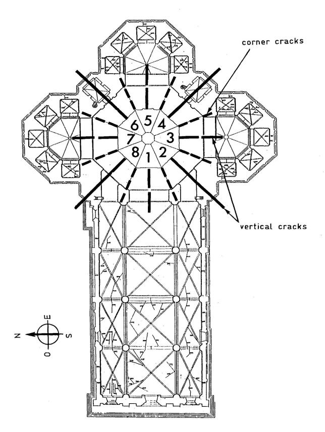
Fig. 1 Plan of the cathedral basement : crack location
