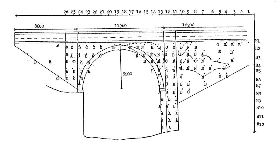
Fig. 2 Bargower Bridge, downstream face, transmission test results.
