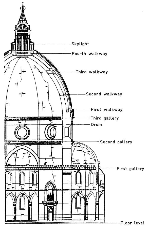
Fig 2 Dome and basement transversal section
