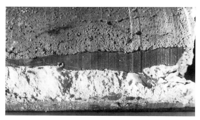
fig. 2 Successful result of grouting. The joint is completely filled. The cement mortar is well interlocked with the porous stone and the lime mortar.
