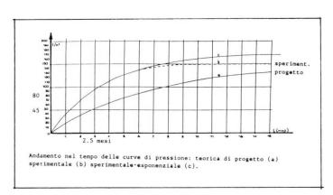
Fig. 6 The evolution of the average pressure with time increasing.
