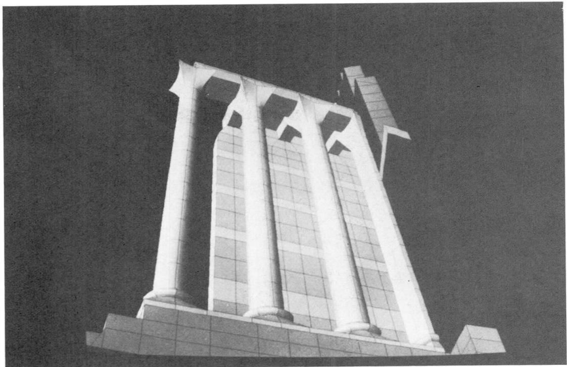
Fig. 3 - 3D F.E. mesh used for numerical simulation of dynamic behaviour for the remains of the Mars Ultor Temple.
