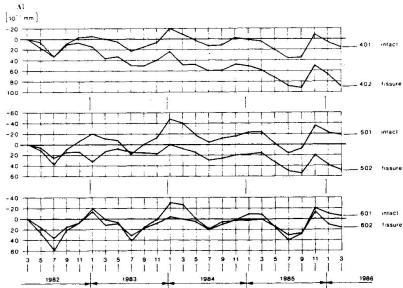
Fig. 3 Evolution of crack-openings
