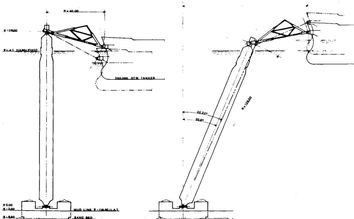
Figure 5 : Single point mooring movements of column, yoke and tanker
