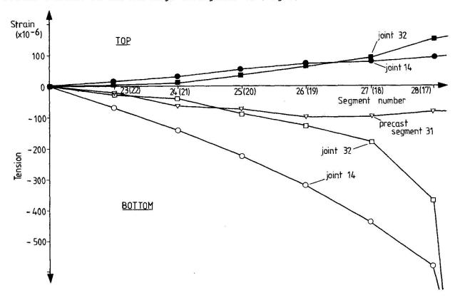
Fig. 3 Comparison of strain changes on south side.
