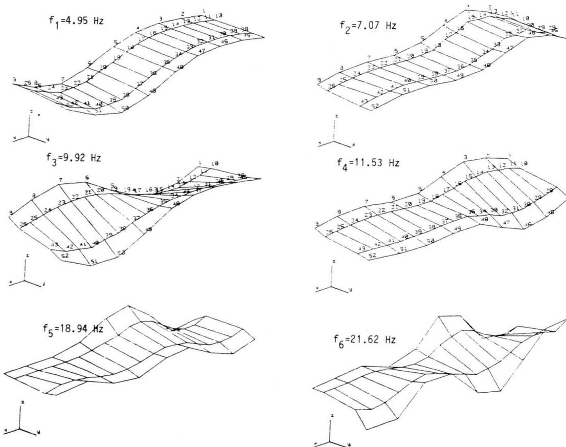
Fig. 4 Mode shapes extracted from the measured response
