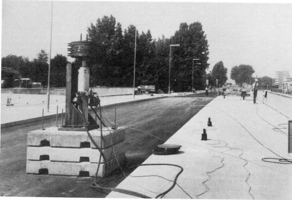
Fig. 3 Bridge Ulenbergstraße, hydraulic exciter (1st measurement)
