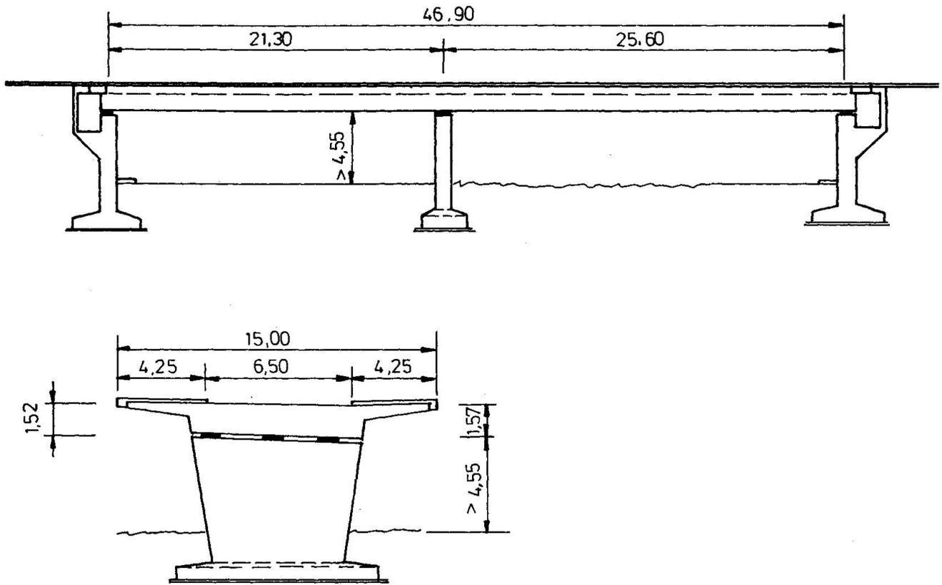
Fig. 1 Bridge Ulenbergstraße, Longitudinal and cross sections
