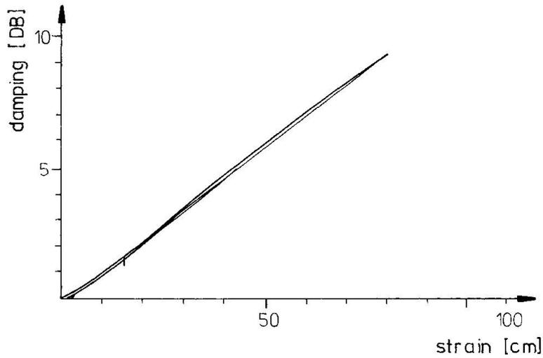
Fig. 6 Damping-strain relationship of the optical sensor
