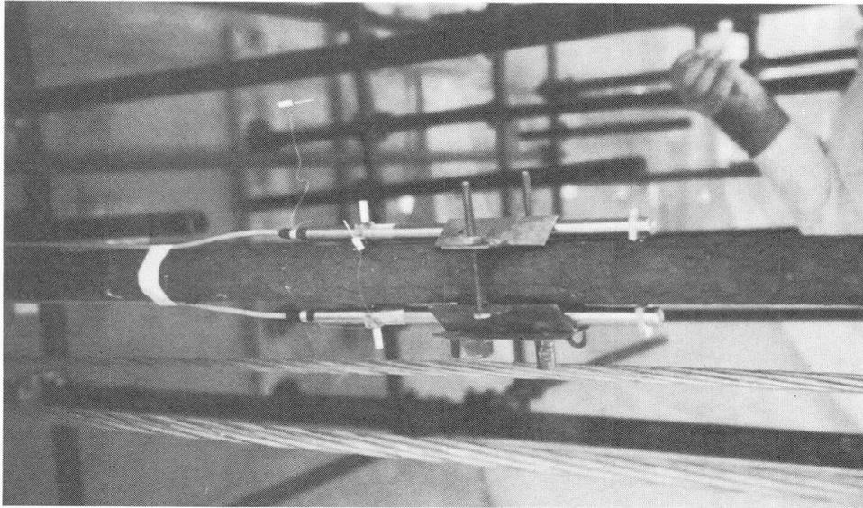
fig. 8 Photo of deformometers applied on a chain for dynamic tests.
