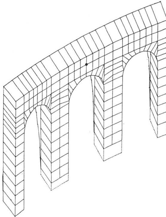
fig. 6 Colosseo: Finite Elements model of the research area.
