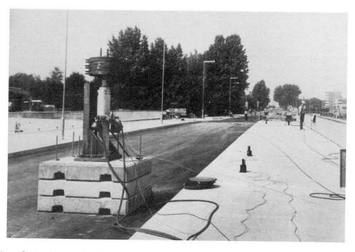
Fig. 3 Bridge Ulenbergstraße, hydraulic exciter (1st measurement)
