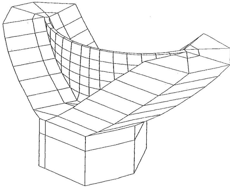
Fig. 3: 3D mesh of the dam and the foundation
