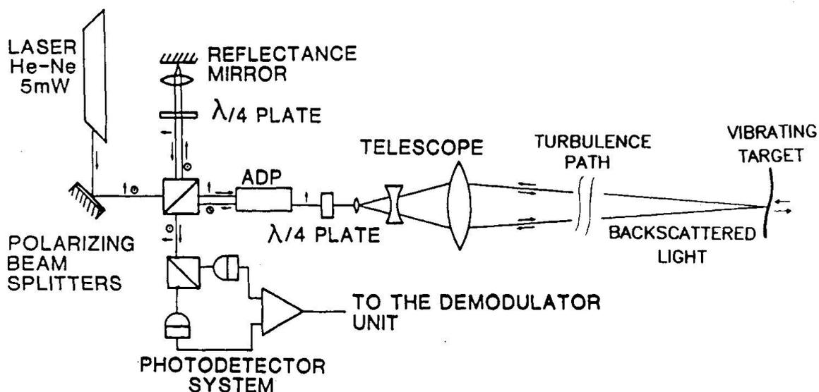
Fig. 1 - Optical set-up of the interferometer.
