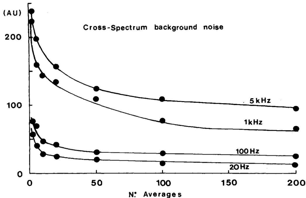
Fig. 3 - Average cross-spectrum of two uncorrelated white noise signals reported as a function of the frequency span of the spectrum analyzer and the number of averages.
