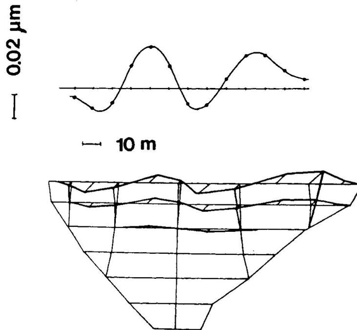
Fig. 10 - The same as Fig. 9 for the first symmetrical mode at 7.6 Hz.
