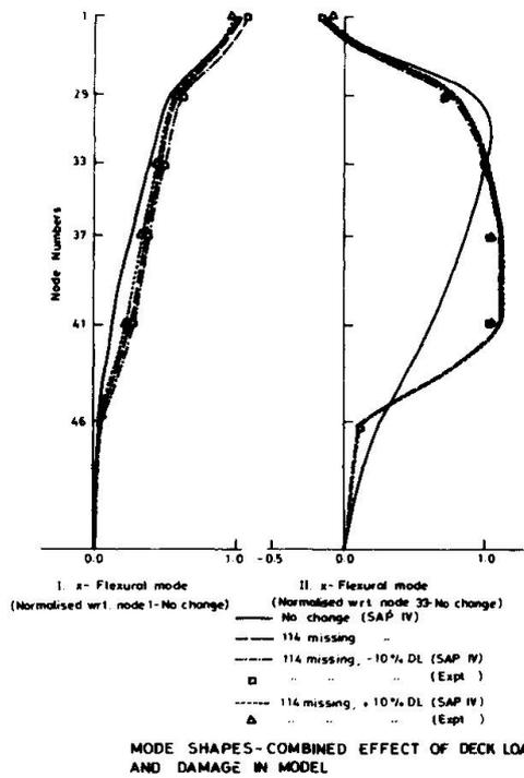
MODE SHAPES-COMBINED EFFECT OF DECK LOAD AND DAMAGE IN MODEL
