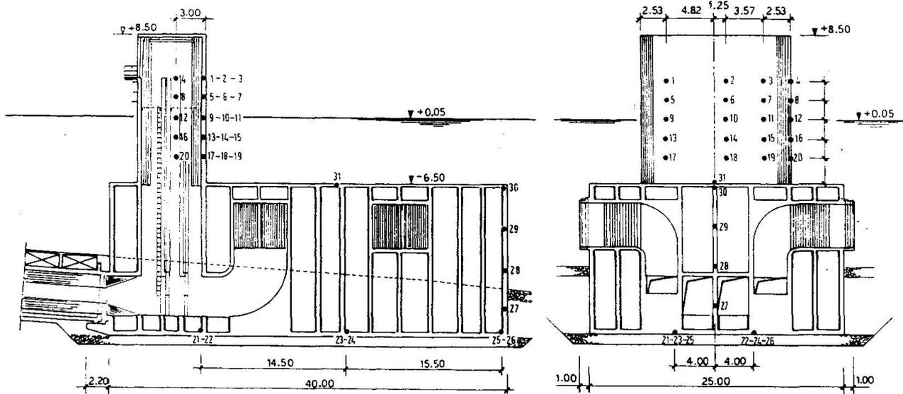
**Fig.9** Torrevaldaliga Nord cooling water intake (lateral and front view).
