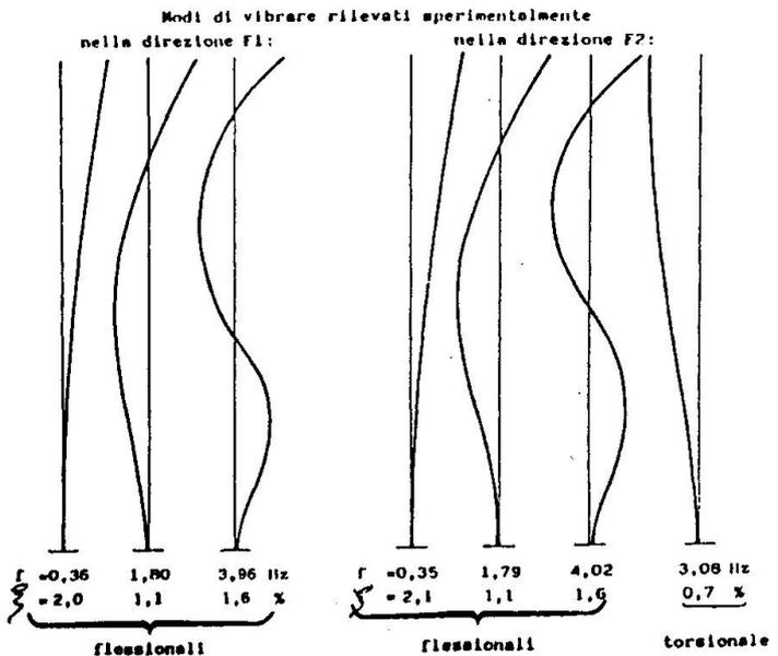
Fig. 7 Experimental modal shapes, frequencies and damping ratios
