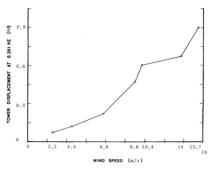
Fig. 7 Tower displacement
