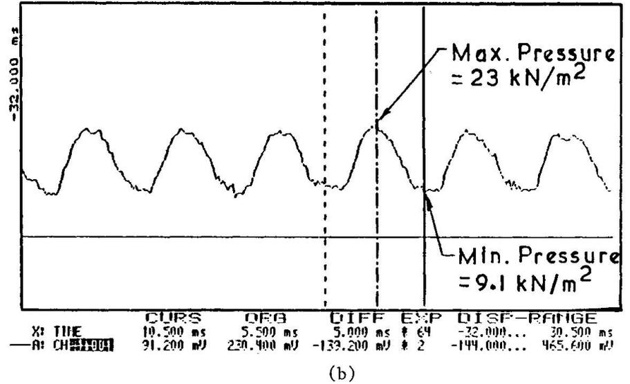
Fig. 12 Results recorded at a mean pressure of 17kN/m<sup>2</sup>
