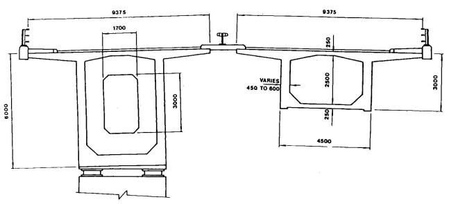
$\underline{\text{Fig. 3(c)}}$  Typical sections through Cogan Viaduct
