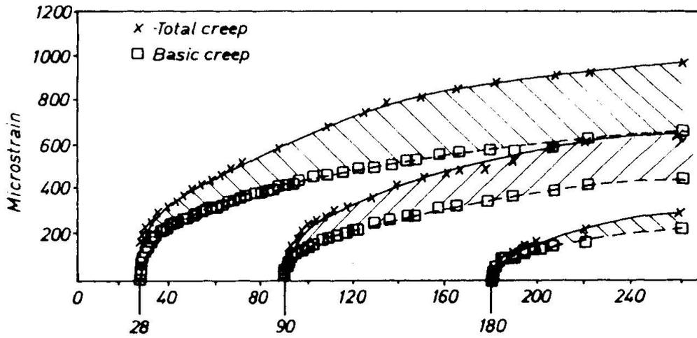
Fig. 9 Typical results from concrete creep tests
