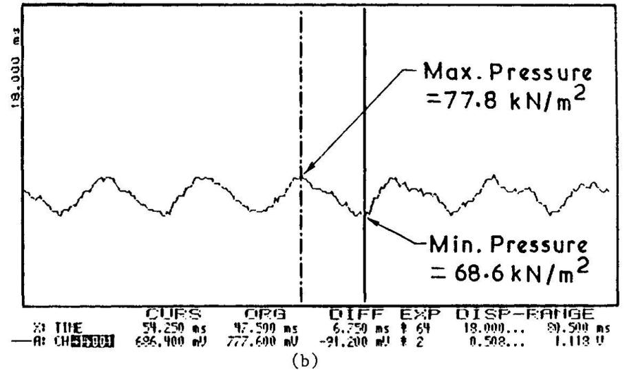
Fig. 13 Results recorded at a mean pressure of 74kN/m<sup>2</sup>
