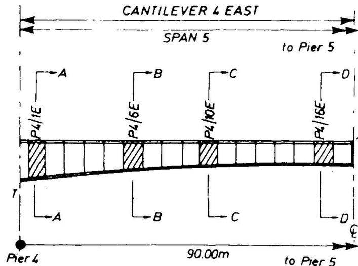
Fig. 4 Instrumented segments
