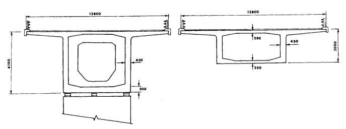
Fig. 3(a) Typical sections through River Torridge Bridge
