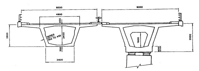
$\underline{\text{Fig. 3(b)}}$  Typical sections through Grangetown Viaduct
