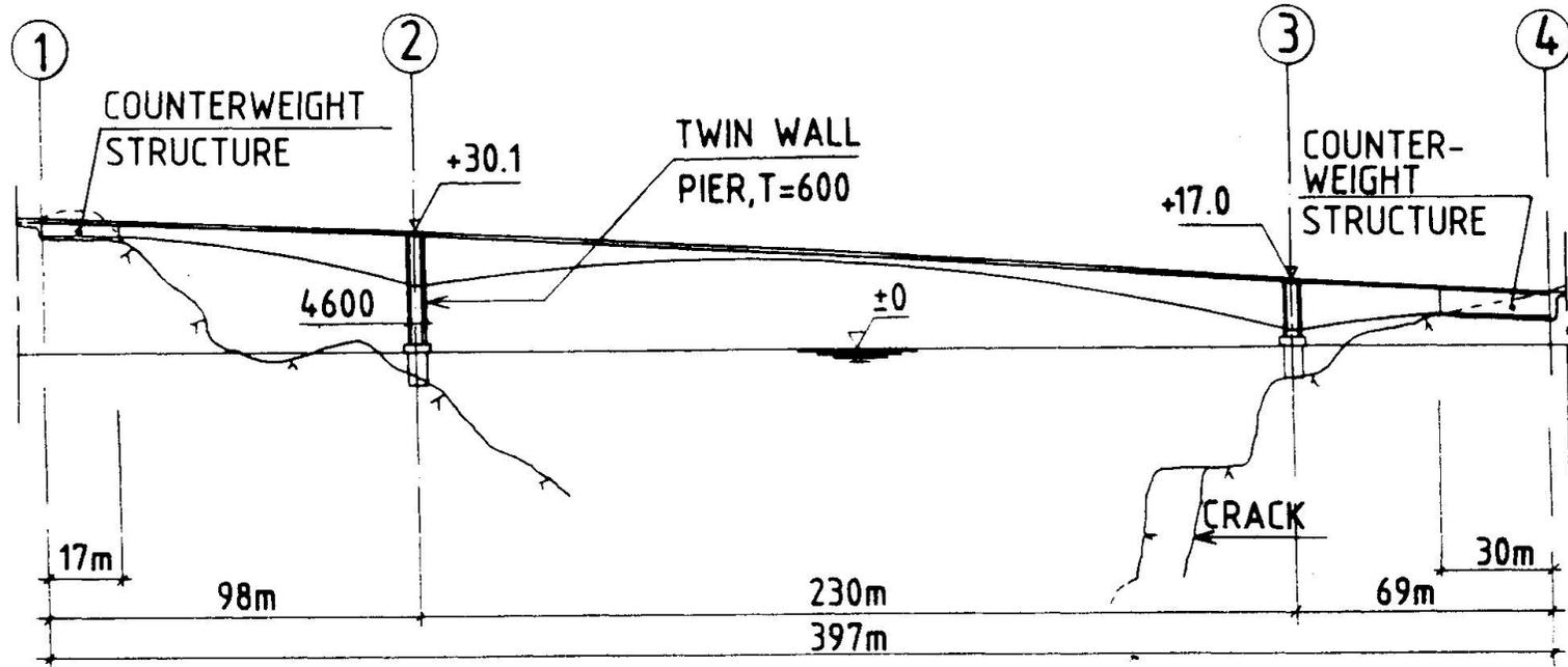
FIG. 1. NORDDALSFJORD BRIDGE. ELEVATION
