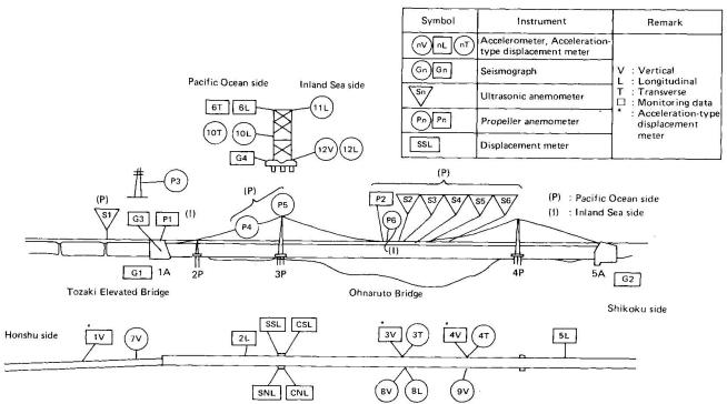
Fig. 4 Arrangement of Measuring Instruments
