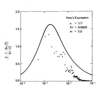
$\frac{f}{U_i} [cycle/m] \label{eq:cycle/m}$  Fig. 6 Power Spectrum of Wind
