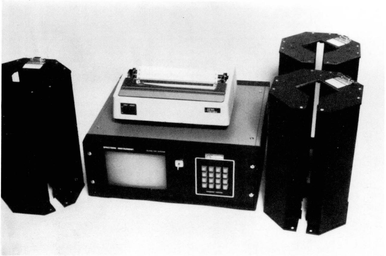
Fig. 2 Plumblin monitoring system
