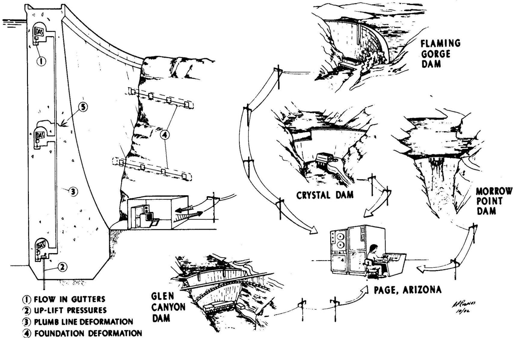
Fig. 1 Schematic drawing of integrated dam monitoring system
