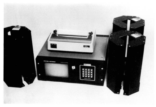
$\frac{\text{Fig. 2}}{\text{prior to installation}} \ \text{Plumbline monitoring system}$
