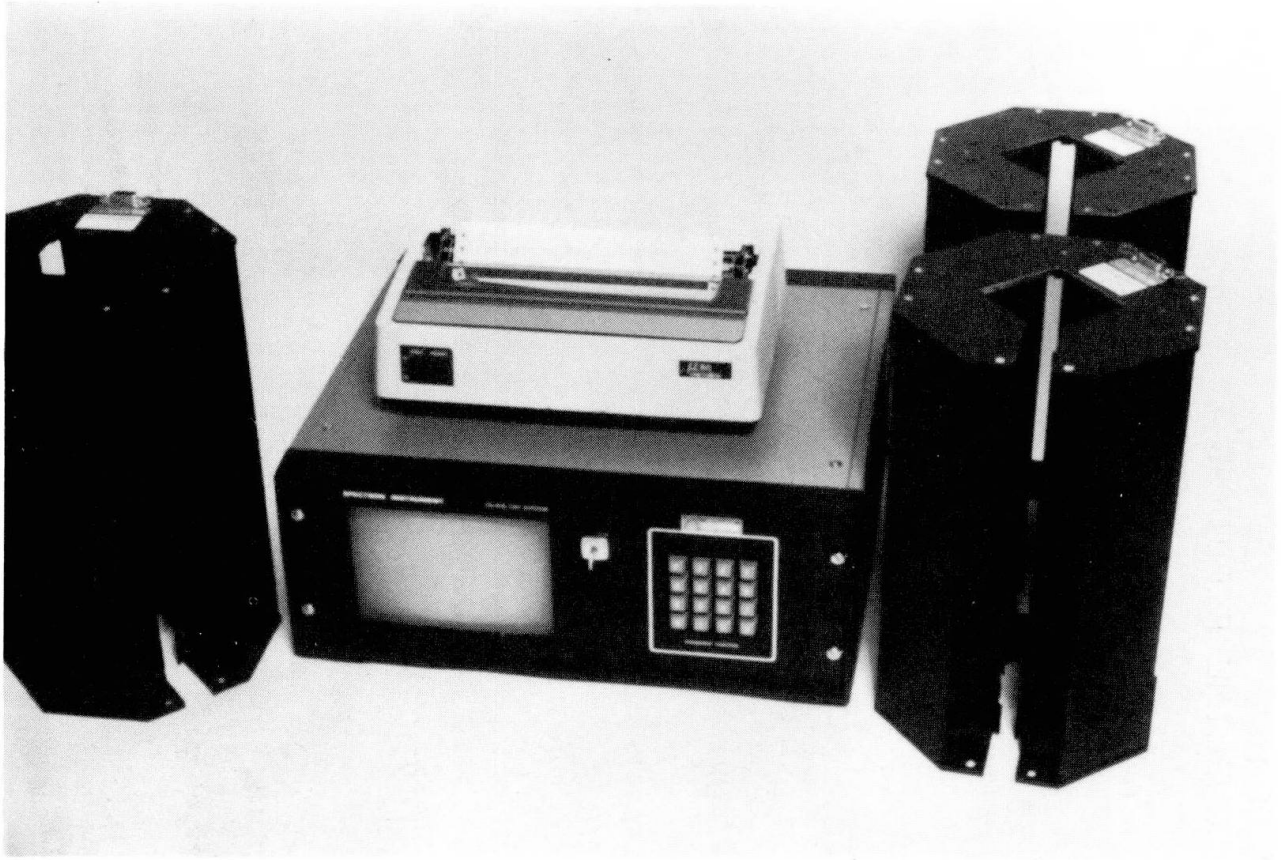
Fig. 2 Plumblin monitoring system prior to installation
