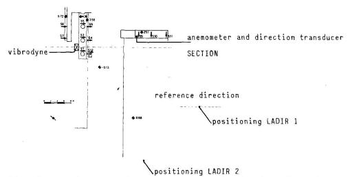
Fig. 4 - Horizontal view of sensors and vibrodyne locations.
