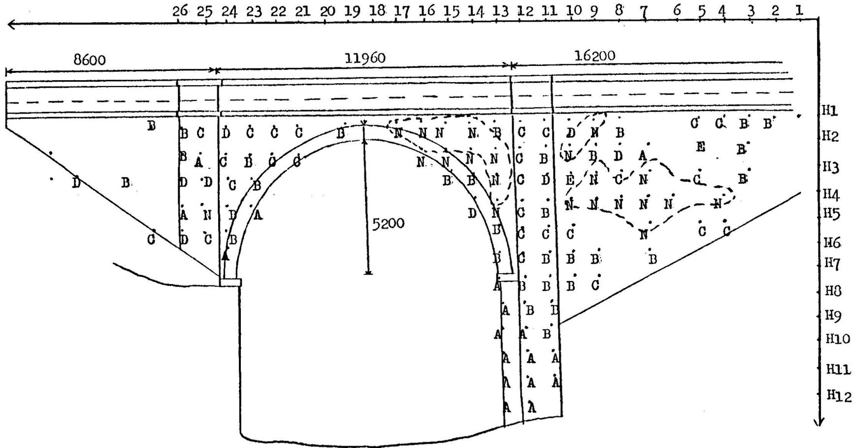
Fig. 2 Bargower Bridge, downstream face, transmission test results.
