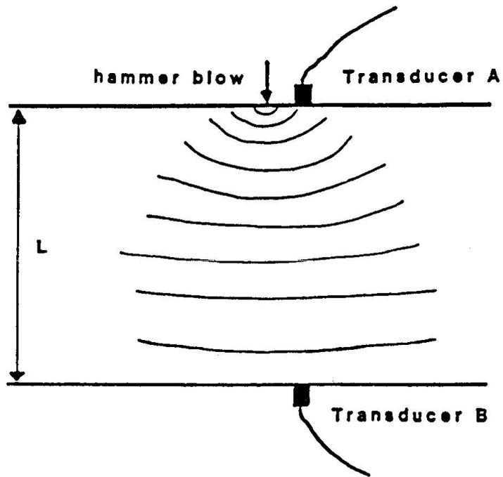
Fig. 1 Time Delay Technique
