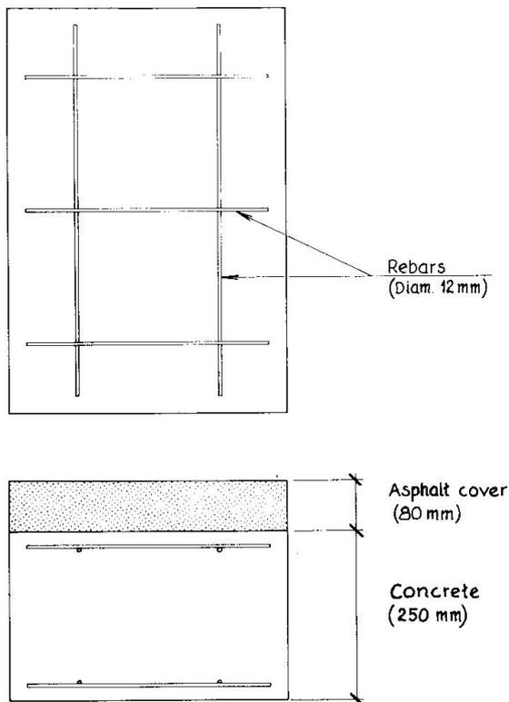
**Fig.2** Test specimen with different chloride ion contents 0, 0.3, 0.6 and 1.2 %, respectively [26].
