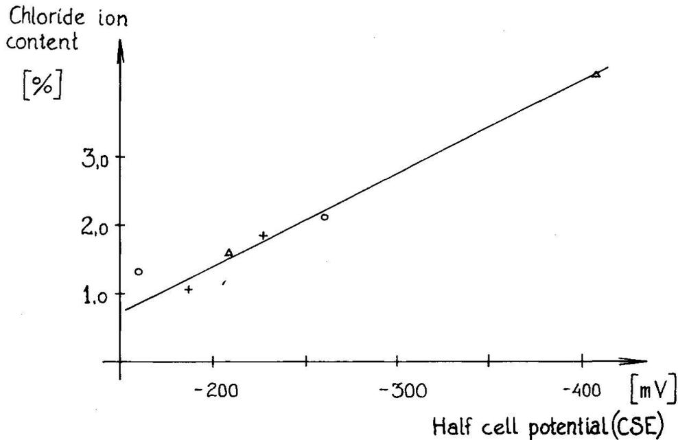
**Fig.1** Observed half-cell potential as a function of the actual chloride ion content [19].
