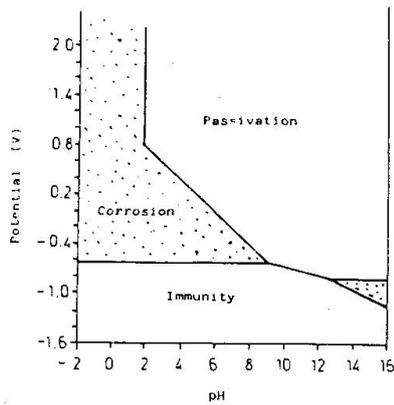
Fig. 1 - Steel corrosion vs. pH value and potential.
