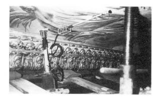
Fig.15 The instruments placed at the intrados of the vault.
