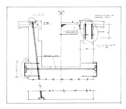
Fig. 27 The intervetions based upon the insertion of prestressed Dywidag bars.
