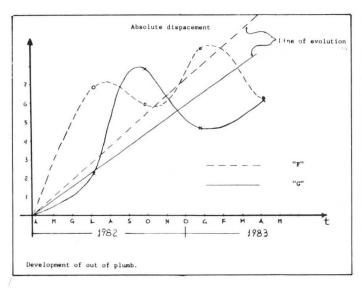
Fig. 23 Development, on time increasing, of the out of plumb of the bell tower.
