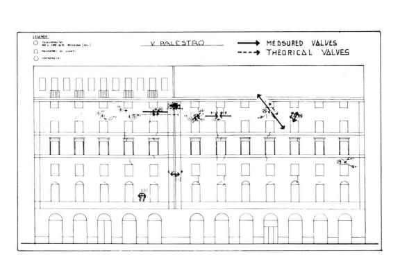
Fig. 31 Comparison between measure of phenomena and the results of theorical analysis.
