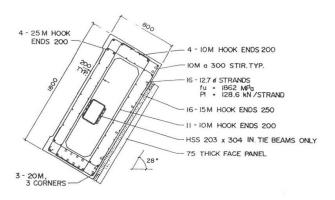
TYPICAL PRECAST CONCRETE PERIMETER BEAM
