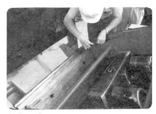
Fig. 5 Checking of mould dimensions
