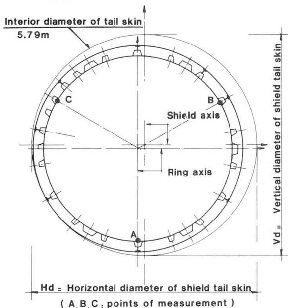
Fig. 6 Eccentricity of ring within the shield machine
