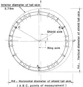
Fig. 6 Excentricity of ring within the shield machine
