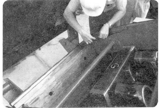
Fig. 5 Checking of mould dimensions
