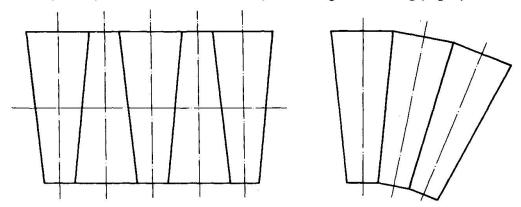
TAPERED RINGS ALIGNED IN STRAIGHT SECTION AND CURVED SECTION
