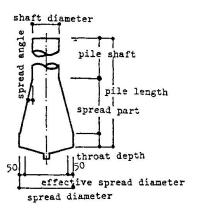
accomplished by augering machine and versatile technique under strict quality control. After confirmation of boring hole geometry by the ultrasonic measuring device the concrete placing can be made under the standardized working chart. By the field experiments with measurement of concrete piles mechanical properties of material tests the present management method is appropriately realised.
