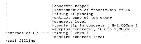
The above work units can be summarized in a form of check sheet, which is filled as the progress of field works. Thus the concrete geometry control can be completed.
