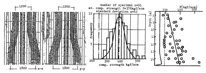
Fig.3 Ultrasonic measurement Fig.4 Histogram Fig.5 F-H relations
