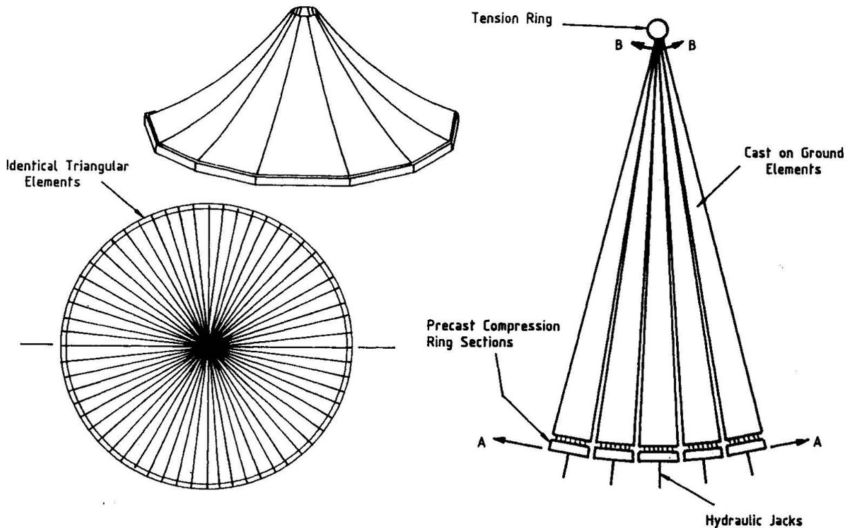
Fig. 7 Conical roof
