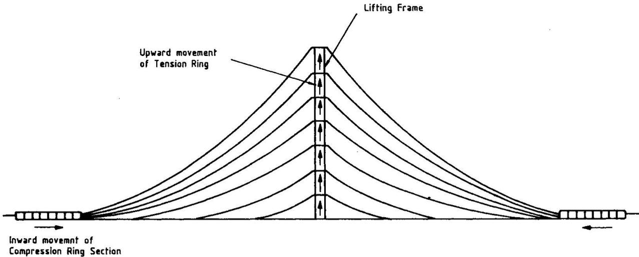
Fig. 6 Progressive lifting of prestressed concrete "tent"
