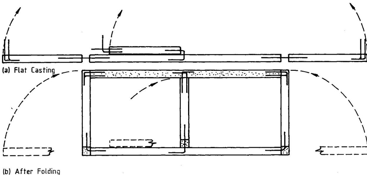
Fig. 3 Box culvert walls "folded" into place
