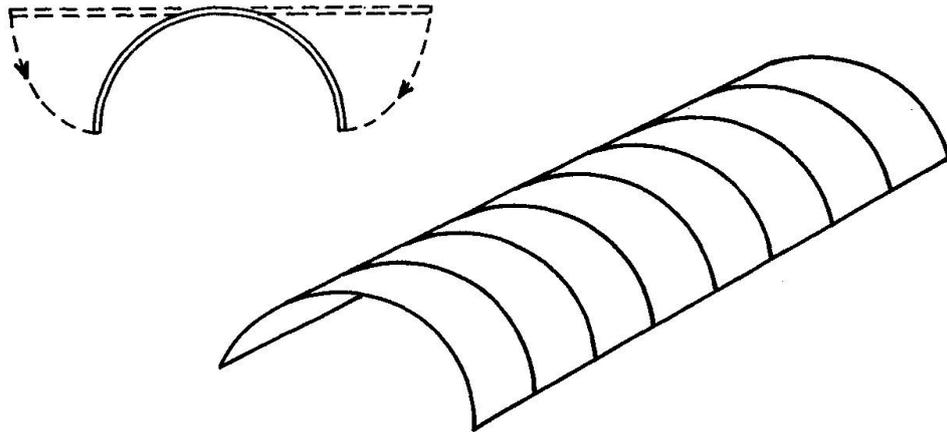
Fig. 5 Barrel vault roof from flat segments
