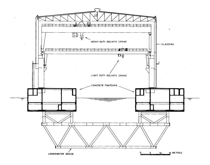
FIGURE 2 - CROSS - SECTION
