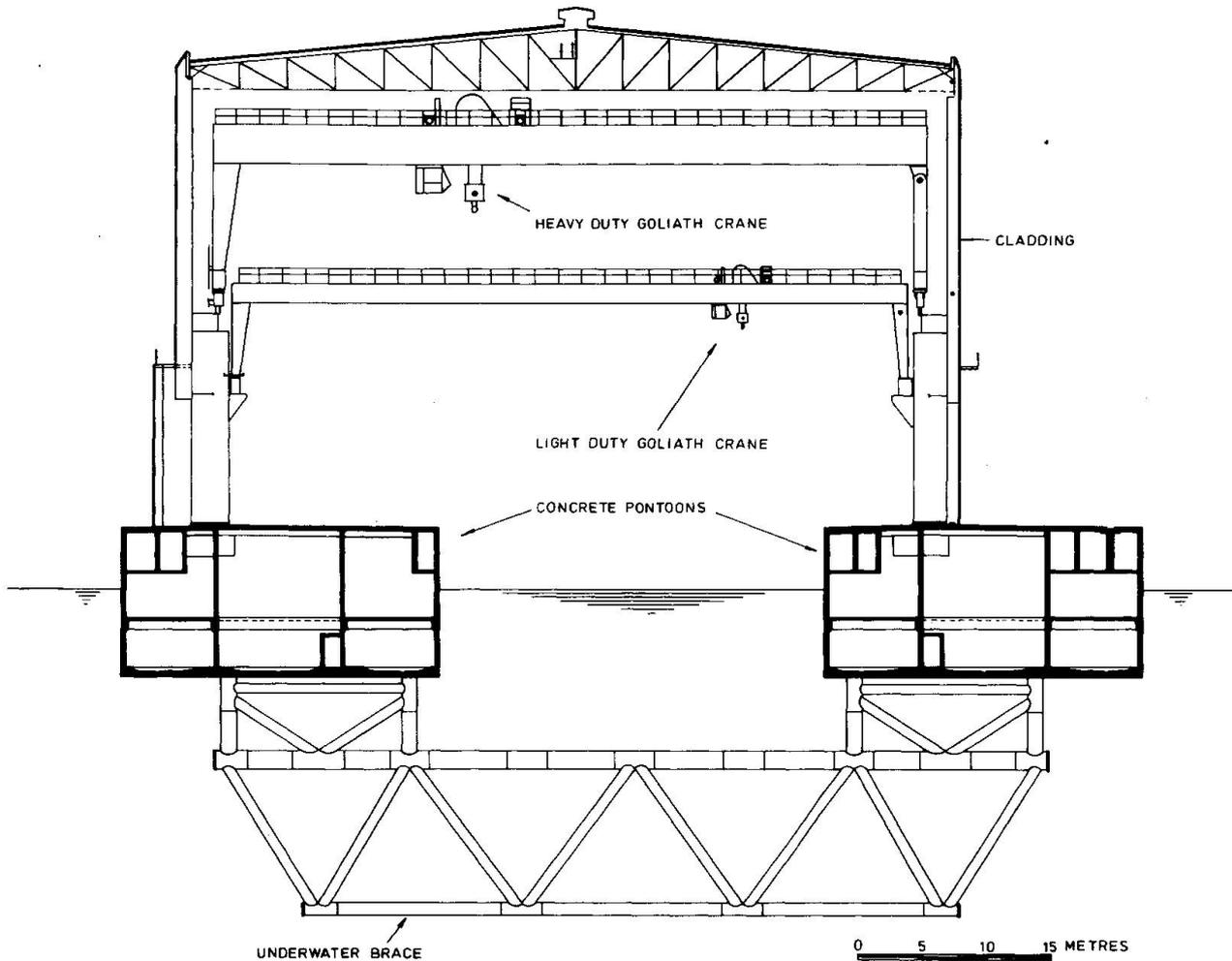
FIGURE 2 - CROSS - SECTION
