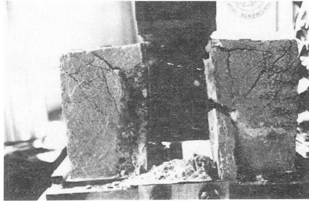
Fig. 7 Failure of specimen B5 under static load
