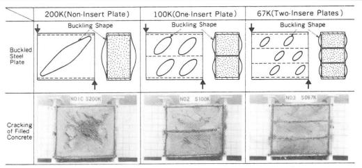
Table 4 Final State of the Steel Plate and the Filled Concrete
