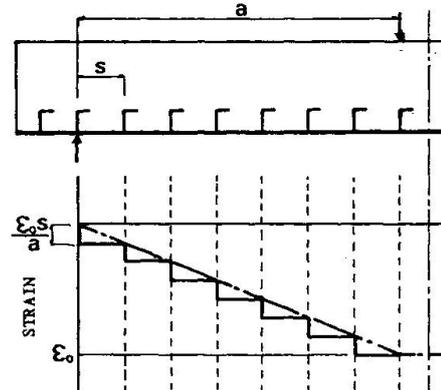
Fig. 6 Axial strain distribution of steel plate
