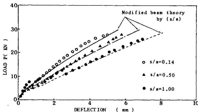
Fig. 5 Load - Deflection curve of composite beam
