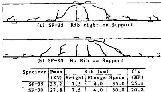
Fig. 4 Effects of rib arrangement on shear strength
