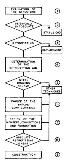
Fig. 7 Flowchart for the retrofitting process [4]
