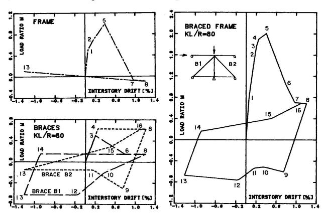
Fig. 5 Frame and bracing system under cyclic loading [4]
