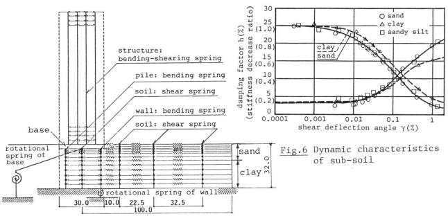
Fig. 5 Modelling in earthquake response analysis
