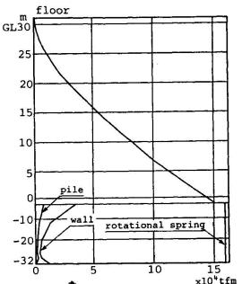
Fig.8 Maximum response overturning moment and bending moment
