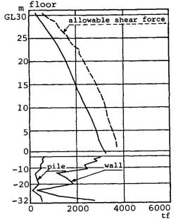
Fig. 7 Maximum response shear force
