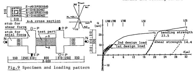
Fig. 10 Load-deflection curve of No.1
