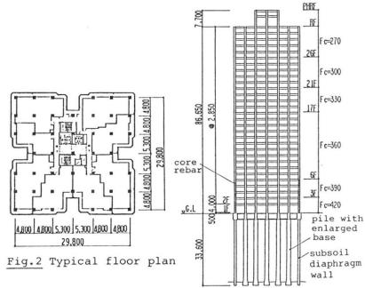
Fig.3 Framing elevation
