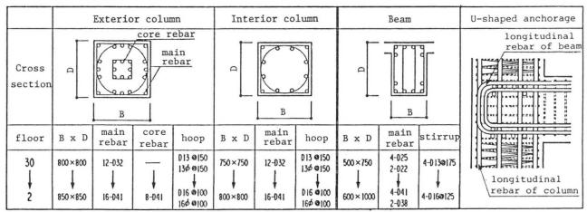
Fig. 4 Typical cross sections
