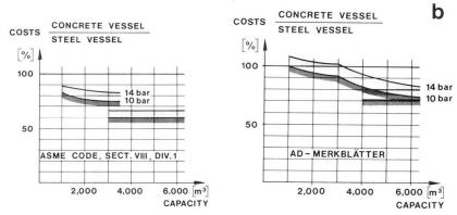
Fig. 3. Costs ratio of spherical pressure vessels
