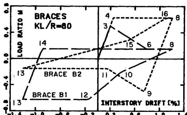
Fig. 5 Frame and bracing system under cyclic loading [4]
