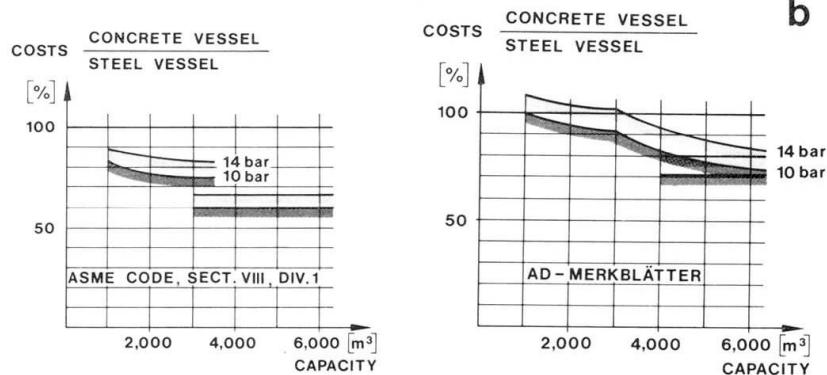
Fig. 3. Costs ratio of spherical pressure vessels
