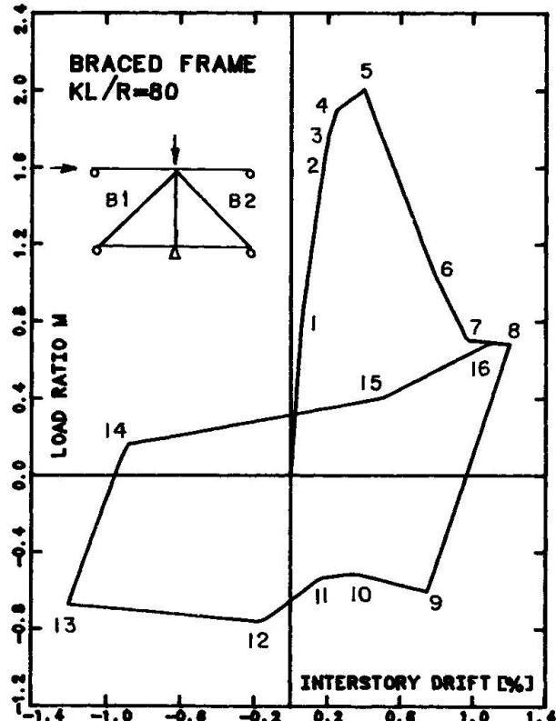
Fig. 6 Braced frame under cyclic loading [4]
