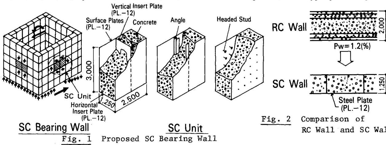
**Fig. 2 Comparison of RC Wall and SC Wall**
