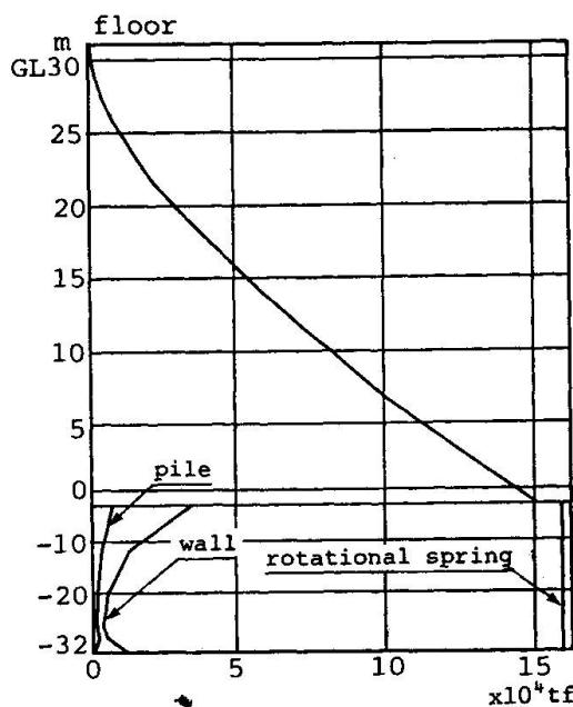
Fig. 8 Maximum response overturning moment and bending moment
