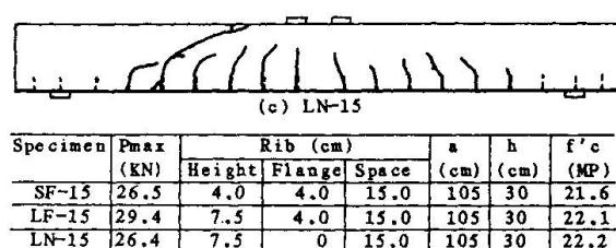
Fig.2 Effects of Rib height and Rib-flange on the strength and composite action
