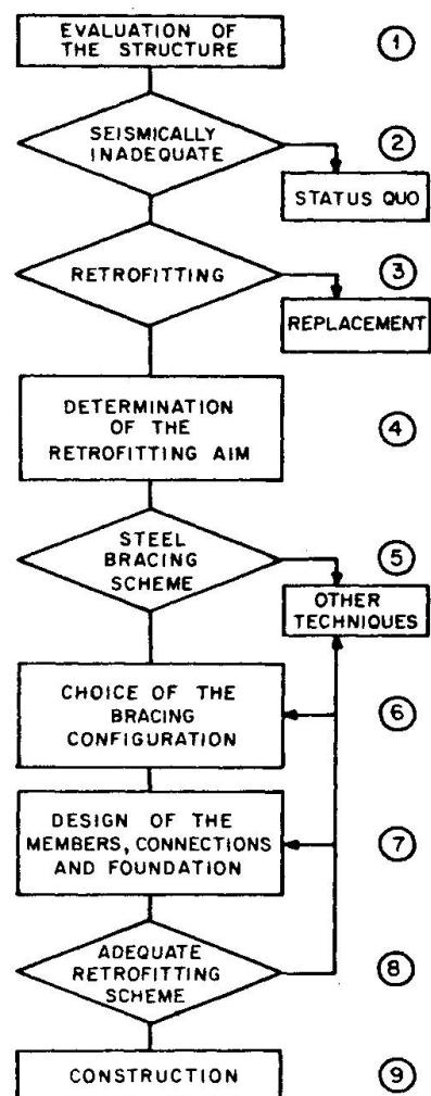
Fig. 7 Flowchart for the retrofitting process [4]
