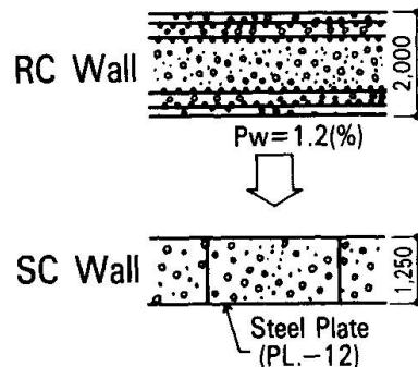
within the unit; 2) stiffen the surface plates by attaching four L-shaped steel angle members instead of the two vertical insert plates; 3) weld headed studs on the surface plates to conform with the AIJ standard for structural design of steel structures (width-thickness ratio  $\leq 41$ )<sup>3)</sup>; etc.
