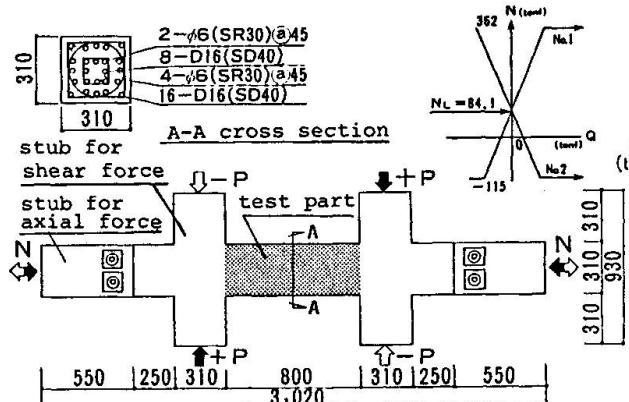
Fig. 9 Specimen and loading pattern
