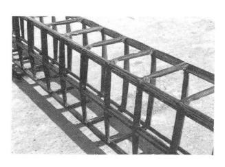
$\begin{array}{c} \underline{\text{Fig. 9}} & \text{Sample of three-dimensional} \\ & \text{shaped NEFMAC} \end{array}$
