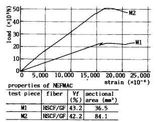
Fig. 2 Schematic stress - strain relationship of NEFMAC
