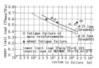
Fig. 10 Fatigue strength of NEFMAC
