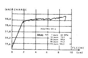
FIGURE 4 - DIAGRAMME CHARGE FLECHE AU CENTRE POUR OK 6
