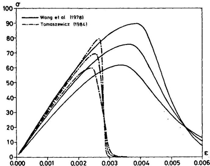
Fig. 1: Stress-strain curves from uniaxial compression tests.
