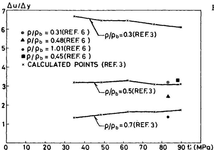
Fig. 2: Relationship between deflection ductility and compressive concrete strength.
