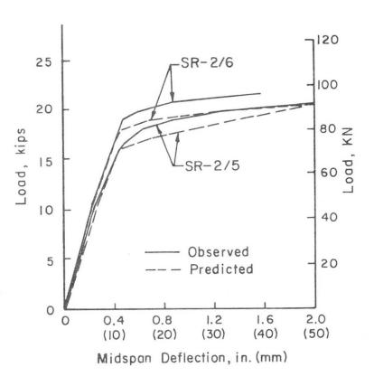
Fig. 2: Load-Deflection Responses for Beams (SR-2/5 has 4.0% steel and SR2/6 has 5.6% steel)
