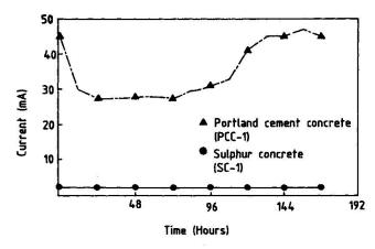
Fig. 3 Variation of current with time in SC and PCC specimens in impressed voltage testing
