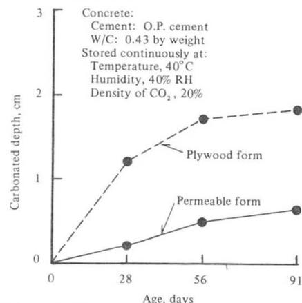
Fig. 7 Comparison of accelerated carbonation test results
