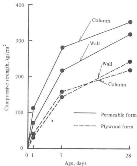
Fig. 6 Comparison of is Schmidt hammer test results
