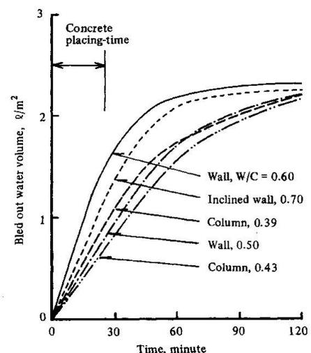
Fig. 4 Water volume bled out from permeable form
