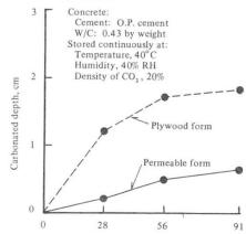
Fig. 7 Comparison of accelerated carbonation test results
