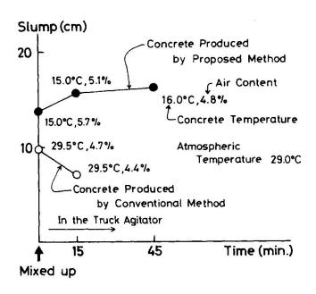
Fig.2 Slump of the concrete produced by proposed method and of conventional concrete
