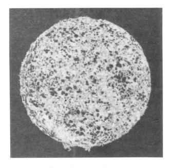
Photo.1 Section of wheat flour and red ink (liquid phase) mixture Photo.2 Section of wheat flour and red ink (frozen and sliced) mixture
