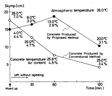
Fig.3 Slump of the concrete produced by proposed method and of conventional concrete
