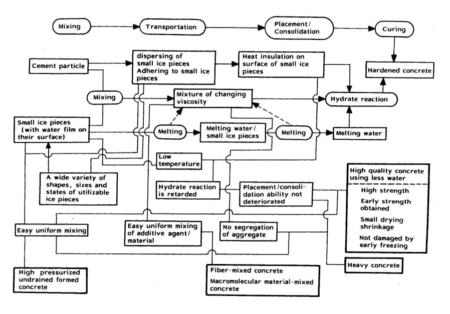
Chart 1 Characteristics of concrete production method utilizing small ice pieces and then melting process
