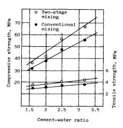
Fig. 4—Compressive and tensile strengths of concrete.
