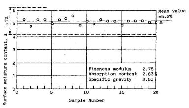
Fig. 7—Control chart of Surface moisture content of sand after adjustment by Sand Controller.
