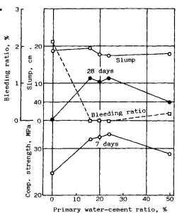
Fig. 3—Primary water-cement ratio and qualities of concrete.
