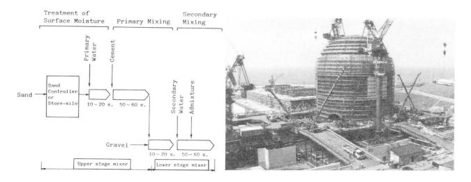
Fig. 8—Flow chart of two-stage mixing method.
