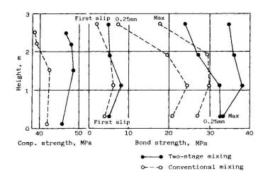
Fig. 5—Distribution of compressive strengths of cocrete and bond strengths of reinforcing steel in wall panels.
