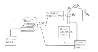
Fig. 4 Control system of concrete distributor
