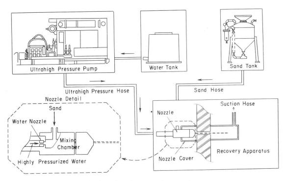
Fig. 9 Scheme of abrasive jet cutting system
