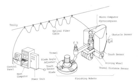
Fig. 5 System of floor surface finishing robot
