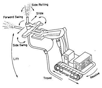
Fig. 2 Movement of shotcreting robot
