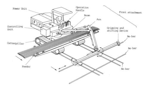
Fig. 7 Scheme of rebar arranging robot system
