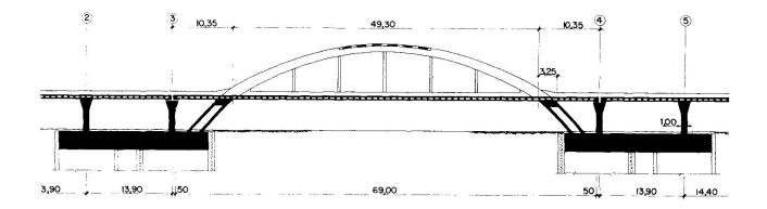
Fig. 1 - Longitudinal section of the bridge.
