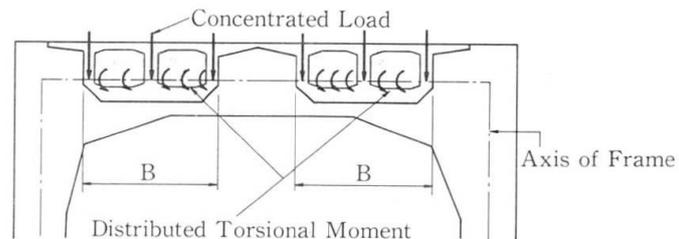
Fig. 11 Loading Condition at Pier
