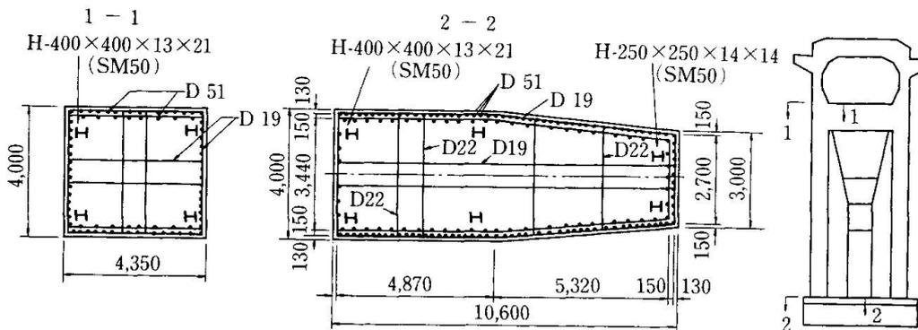
Fig. 6 Cross Section of Pier (6P)
