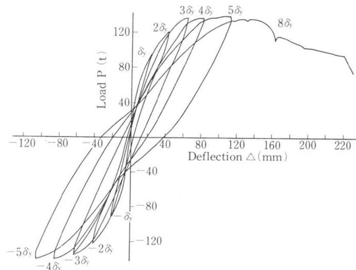
Fig. 10 Relation of Load-Horizontal Deflection at Upper Beam
