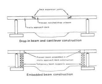
Fig. 4 Precast Beam Deck Continuity Fig. 5 Avoiding Half-Joints
