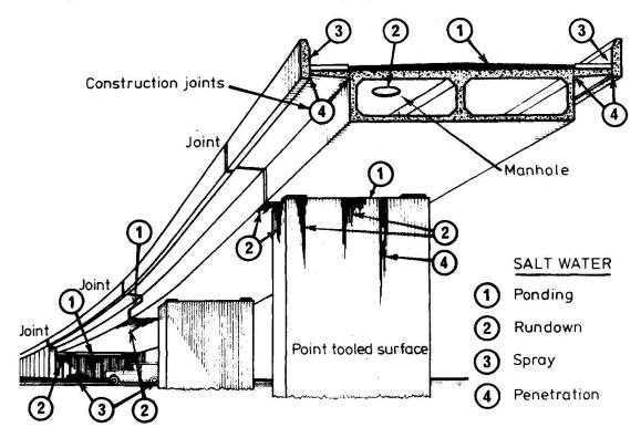
Fig. 3 Typical Salt-Vulnerable Zones
