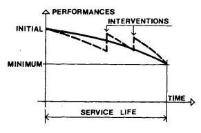
Fig. 1. SERVICE LIFE OF CONCRETE STRUCTURES
